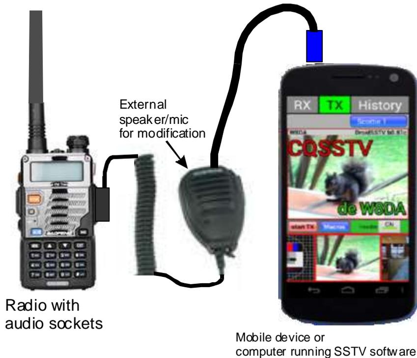
**Figure 5 Wiring to allow reception and transmission of SSTV**
