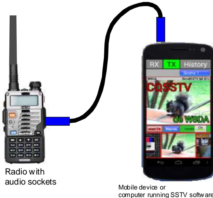
**Figure 2 Minimal equipment setup for receive only**
