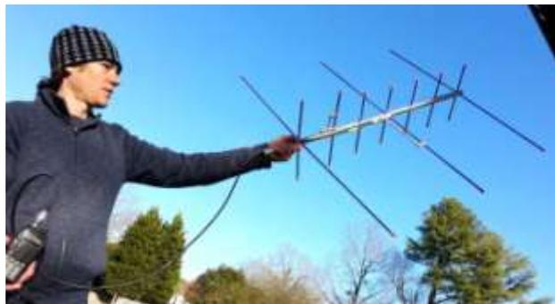
Figure 3 A dual band Yagi for use with satellites
